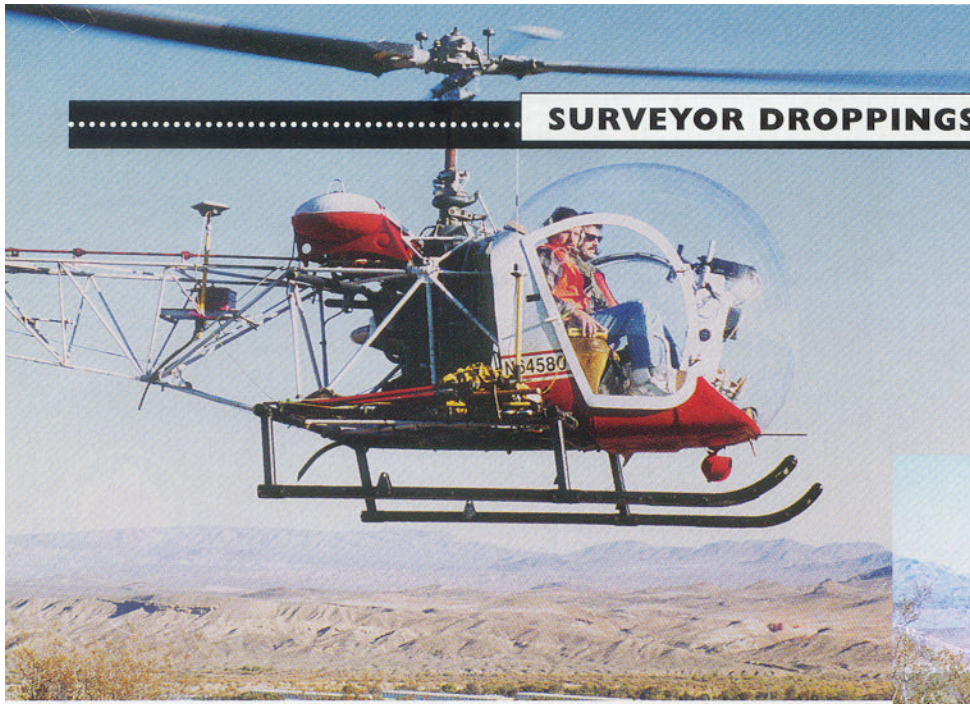
(left) Helicopter with RTK GPS mounted and operating for section corner search. (below) Stone Mound Section Corner.
